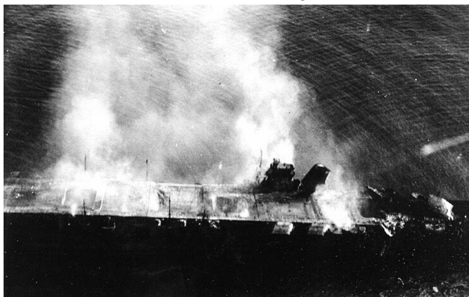
ANOTHER VIEW of the burning Hiryu , taken early in the morning of 5 June. Bombs exploding on her hangar deck along with planes being refueled and rearmed, collapsed the flight deck forward of the island and threw a portion of the forward elevator against the island, where it stayed.
