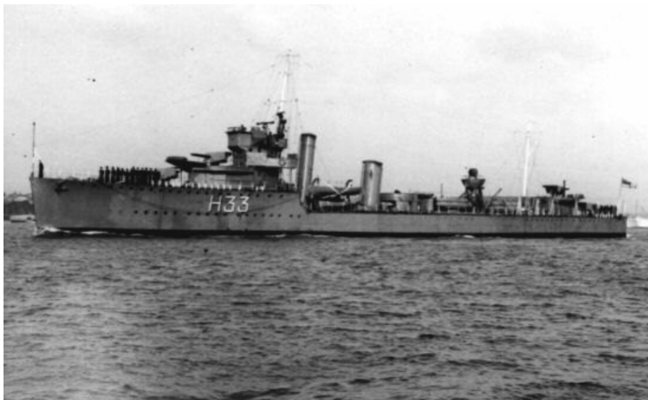
HMS Vanoc, a first war destroyer that had been fitted with an early form of radar just prior to the escort duty during which she sank Joachim Schepke's U-100. Her detection of Schepke when he surfaced was the first known instance of a radar bearing on an enemy by a surface warship.
